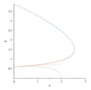
**Fig. 7.** Eigenfrequencies  $\omega$  as functions of the load parameter p: highest eigenfrequency of the free system (dashed green), lowest eigenfrequency of the free system (plain red), optimal constrained system (dotted blue) and fixed (p=0) constrained system (mixed dashed-dotted gold): the optimal constraint curve is lower than the fixed constraint curve.(For interpretation of the references to colour in this figure legend, the reader is referred to the web version of this article.)
