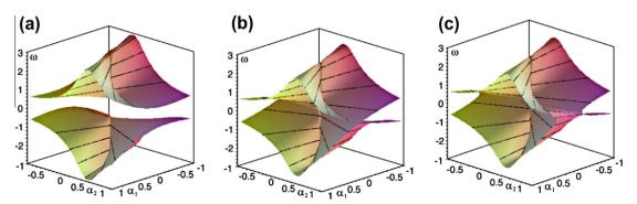
**Fig. 9.** In the  $(\alpha_1, \alpha_2, \omega_{cons})$  space the surfaces of frequencies of the constrained system plotted for (a) p = 1.5, (a) p = 2.1.
