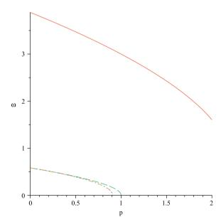
**Fig. 6.** Eigenfrequencies  $\omega$  as functions of the load parameter p: lowest eigenfrequency of the free system (dashed green), highest eigenfrequency of the free system (plain red), optimal constrained system (dotted blue) and fixed (p=0) constrained system (mixed dashed-dotted gold): the optimal constraint and the fixed constraint give the same curve.(For interpretation of the references to colour in this figure legend, the reader is referred to the web version of this article.)
